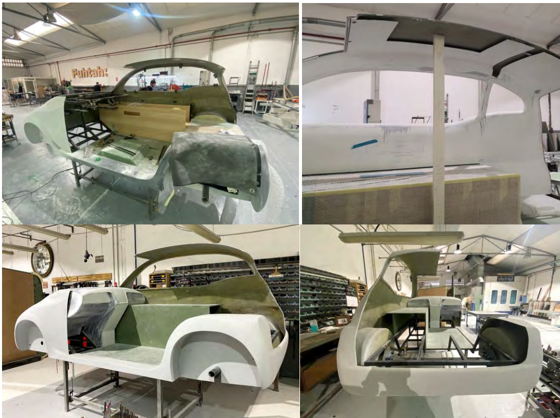
Figure 16: Assembly of the body and dashboard to the tubular structure
