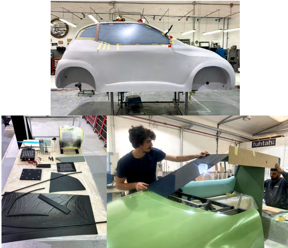
Figure 24: Window fixation process on the mockup
