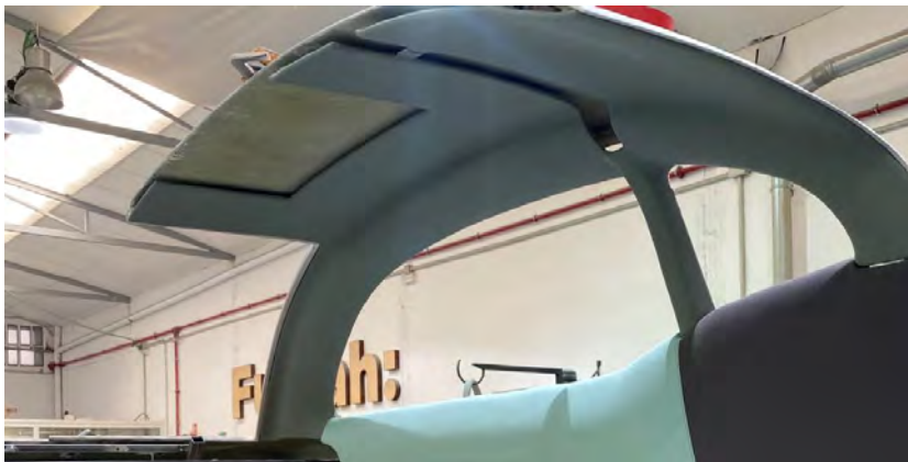
Figure 9: Insulation panel provided by HUT and installed on the Roof
