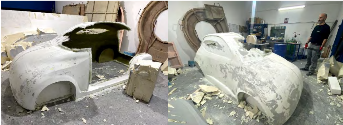
Figure 15: Fiberglass body made from a milled polyurethane mould.
