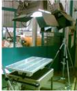
Picture 8: Setup for the test of photovoltaic panels
