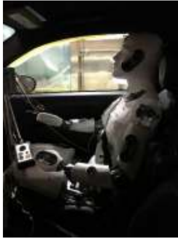
Picture 9: Proprietary Thermal Comfort Manikin P. A. C. O.
