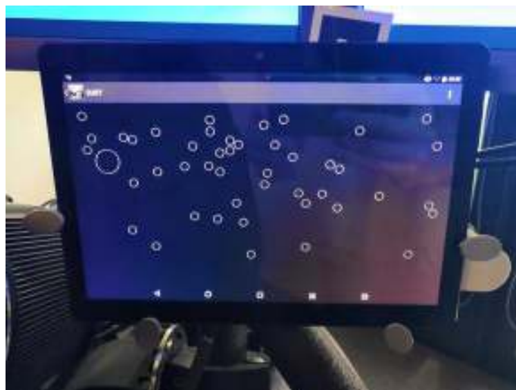
Picture 14: SuRT - The drivers select the left side of the display where the large circle is located
