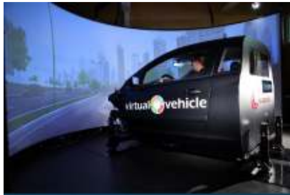
Picture 13: Driving simulator used in the study
